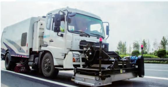
Iron suction vehicle (independently developed by Shaoxing Management Centre) operated in the “Expressway Spillage Special Rectification Action” to effectively prevent tire puncture due to iron nails and other sharp objects.
