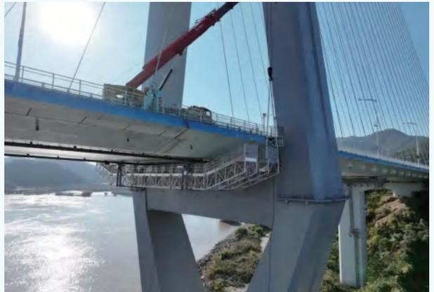
Zhoushan Management Centre put into use a new type of girder bottom inspection vehicle at the Taoyaoamen Bridge, which adopts fully automatic control and has the characteristics of accuracy, safety, environmental protection, no noise and no pollution.
